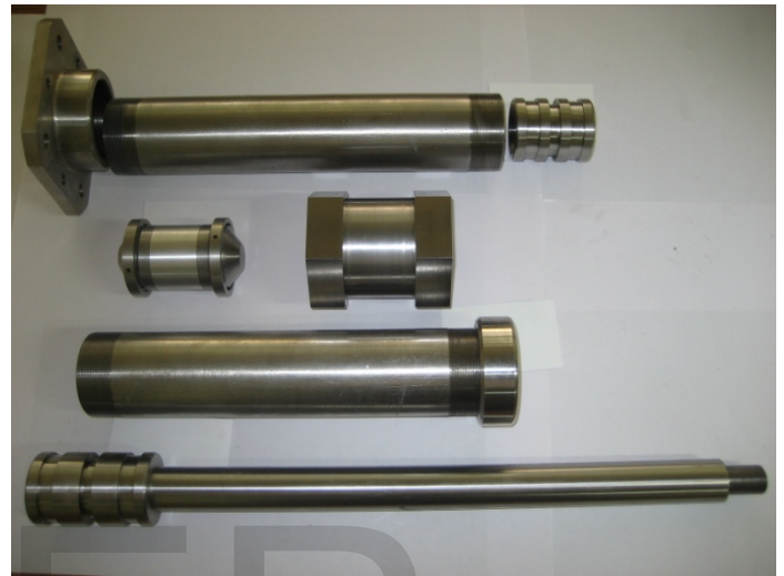
Fig. 6. Machined parts for landing gear assembly
